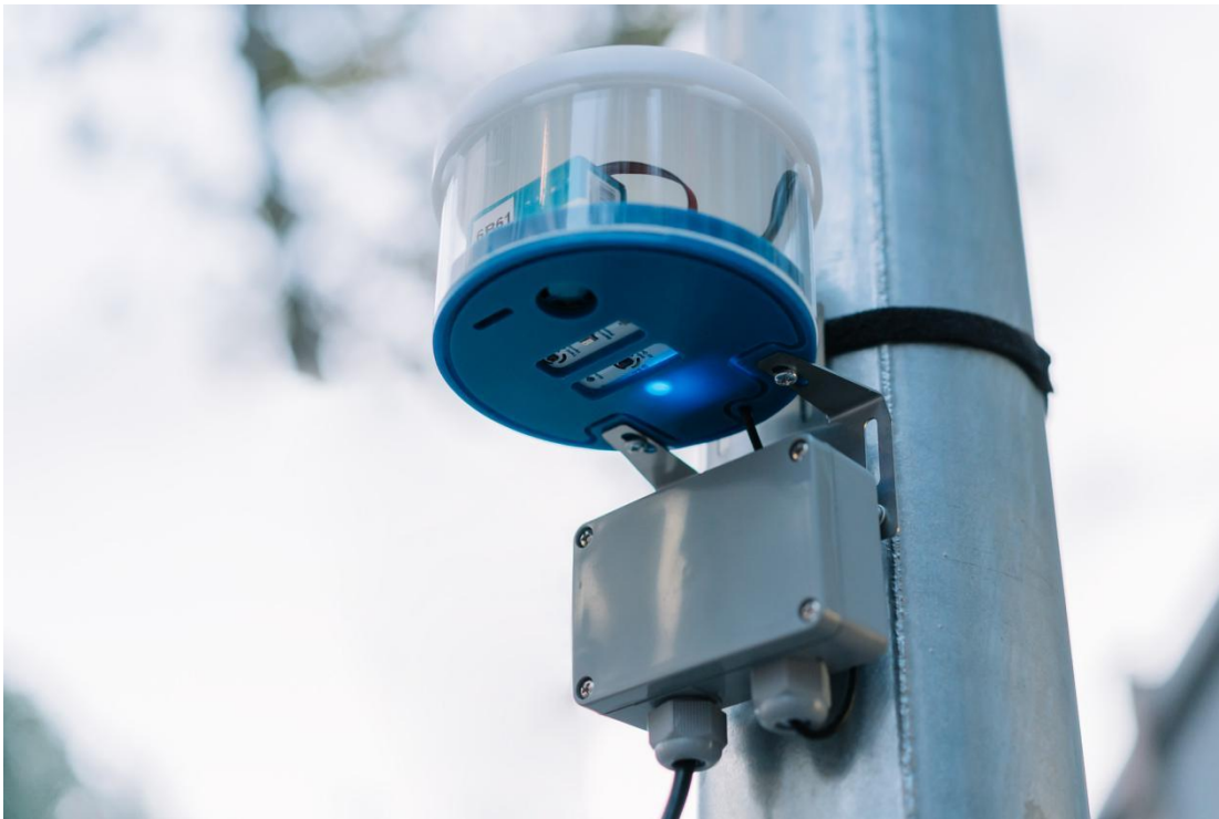
Fig. 7: The deployed outdoor Air pollution monitoring system using the Smart Citizen Kit infrastructure (Source: Smartcitizen, 2025)
